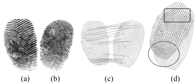
Fig. 1. Example of large distortion from FVC2004 DB1. (a) 102_3.tif, (b) 102_5.tif, and (c) the map relations of the corresponding minutiae in fingerprint images 102_3 and 102_5, (d) the image is fingerprint 102_5 (after registration) added to 102_3. In the rectangle region, the corresponding minutiae are approximately overlapped. While in the ellipse region, the maximal vertical difference of corresponding minutiae is more than 100 pixels.
